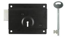
A low security lock commonly fitted to shed and green house doors which is surface mounted for quick and easy installation. The lock bolt engages on or into the door frame and does not require a keep.
