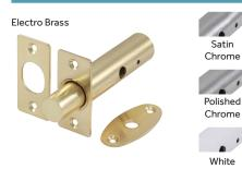
An ideal way to increase security on timber doors. Morticed into the door and operated by a spline key that throws the bolt into the frame. For optimum security its recommended that the bolts are fitted to the top and the bottom of the door.
