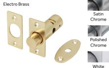
An ideal way to increase security on timber windows. Morticed into the window and operated by a spline key that throws the bolt into the frame. For optimum security it is recommended that the bolts are fitted to the top and the bottom of the window.
