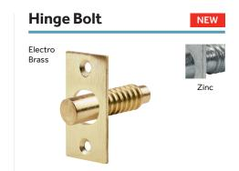
Hinge bolts provide additional security for outward opening doors that have exposed hinge knuckles. They prevent the door being removed from the frame in the event of the hinge knuckle being attacked by interlocking the door into the frame.
