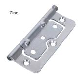
Hurlinges enable quick door fitting as they require no morticing into the door or frame. They feature lugs on the knuckle for quick and simple lining up. The hinge features a removable pin to enable quick door hanging and removal at a later date.
