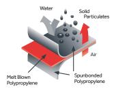
SMS triple layer fabric for enhanced protection
