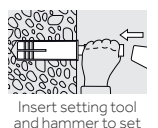
Insert setting tool and hammer to set
