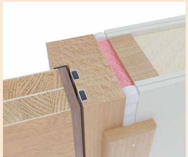
Image B – Intumescent sealant with Fire & Acoustic Seals Fire Door Foam™ for joint widths up to 25mm to achieve ratings of up to 120 minutes when applied correctly.
