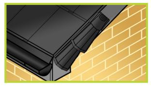
5. Slide the next verge unit into the upper edge of the first unit and press firmly to the tile, fitting it under the head laps to ensure the unit is firmly held in place and then locate the unit through the top grid into the batten.
