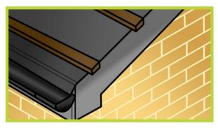
1. Install the tile battens with a 50mm overhang over the brick or barge board. Remove existing mortar bedding in refurbishment projects and install new tiling batten to the underside of the existing tiling batten.
