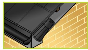
4. Slide the first verge unit over the tile at the eaves and locate into the starter kit, fitting under the head laps to ensure the unit is firmly held in place. Screw the unit through the top grid into the batten.
