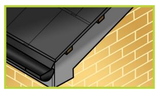
2. Lay tiles and set flush with the battens. Remove existing mortar bedding in refurbishment projects and install new tiling batten to the underside of the existing tiling batten.
