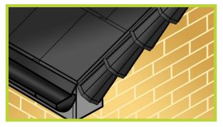
6. Continue the process along the barge board up to the ridge. If required insert the blanking plate over the final verge attach the grid to prevent water ingress. When the other side verge is completed to the apex, secure the ridge end cap to the ridge batten.
