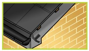
3. Starting at the bottom edge of the roof insert the starter piece into the front edge of the verge unit and mark out the starter piece position on the facia and barge board. Remove the unit and mechanically fix the starter piece in position through the grid.
