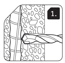
When rebar is encountered, while drilling with a hammer and carbide hammer bit, immediately stop and remove the bit from the hole (failure to do this will severely damage a carbide hammer bit).
