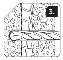
Remove the rotary rebar cutter after the rebar has been drilled completely through and finish drilling the hole with a hammer bit.
