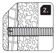
With a rotary rebar cutter mounted in the drill ensuring it is in the rotary-only position. Insert the rotary rebar cutter into the hole and drill through the embedded rebar.
