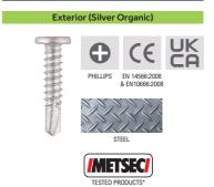
A medium duty metal to metal screw with a large flat surface under the head, making it ideal for fixing thinner sheet material when a flush finish is required. Silver organic plated to withstand over 500 hours salt spray test.
