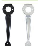
**Technical Data** Size (mm) 200 To Suit Cylinder Ø (mm) 26 Length (mm) 200 Length (inch) 8 No. of Screw Holes 3 Screw Ø (mm) 3.5 A high quality pull handle to suit the extended throw locks. The pull handle fits over the rim cylinder of the lock to provide a clean finish to the cylinder hole.
