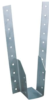
Designed to give a quick and simple solution for various timber connections such as joists and stairwell trimmings. Increased leg lengths, all widths can take up to a 225mm deep joist.
