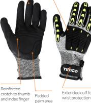
Designed to combat hand and finger injuries specifically in industries with high risk of crushing impact hazards. Fitted with strategically placed TPR segments to help prevent damage to back of hand and fingers. Cut resistant liner and longer, fastening cuffs for wrist protection and comfort.
